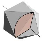
**Figure 10.22.** The icosahedron permits a one-third turn of any face.
